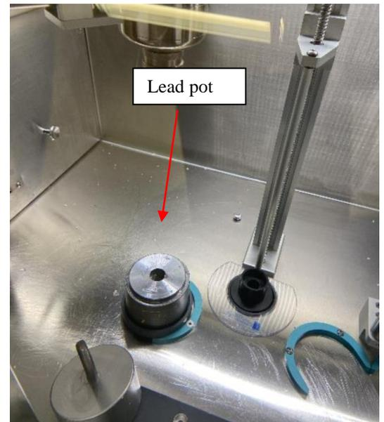
Figure 3: Lead Pot Containing Broken vial inside the shielded box
