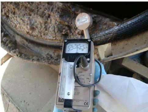
Survey meter detecting NORM in the sludge of a contaminated vac truck
