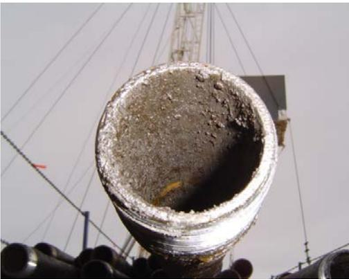
Pipeline contaminated with NORM
