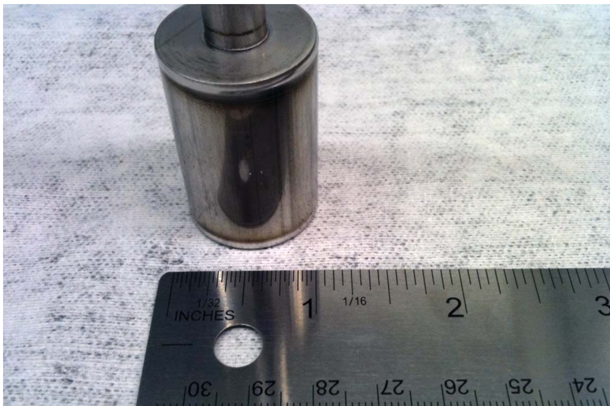
This is an example of a typical tritium bed. It contains the tritium that is used in the production of GTLS.
