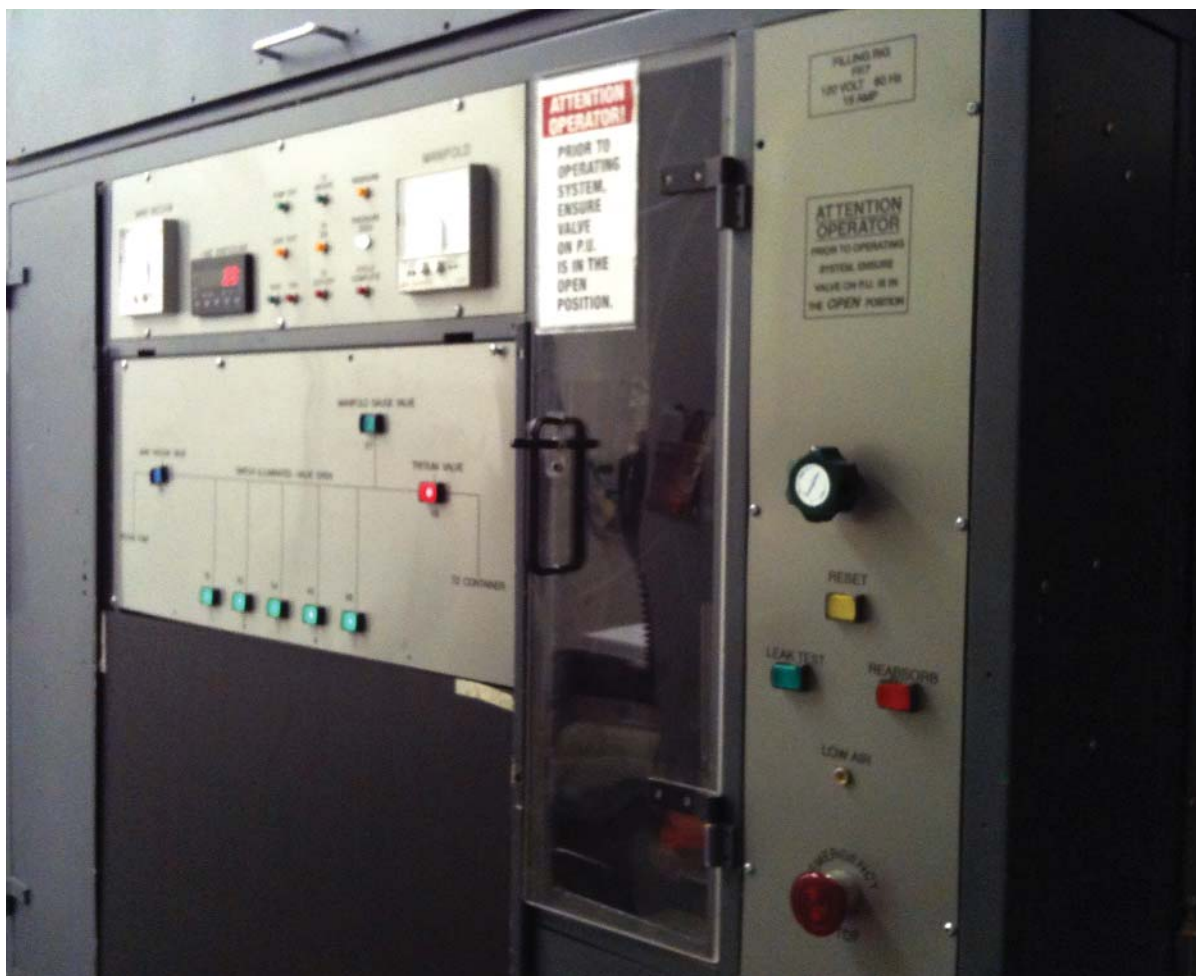
A typical filling rig is used to fill glass tubes with tritium gas at a gaseous tritium light source facility.
