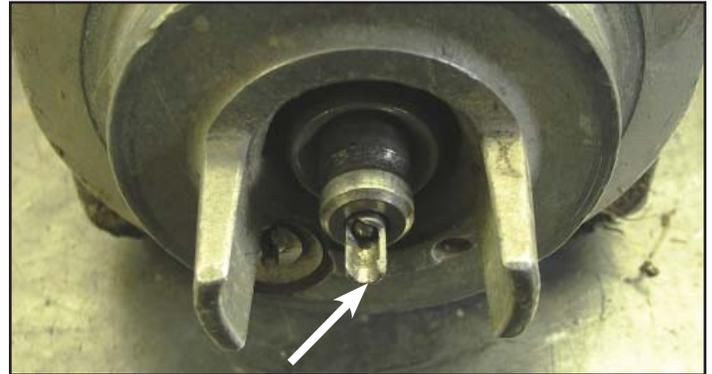
*Two incidents involving the source assembly in MDS Nordion Gammamat TSI 5/1 exposure devices were reported to the CNSC. In each case, the female connector on the source assembly broke in half while the source assembly was in the fully shielded position.*
