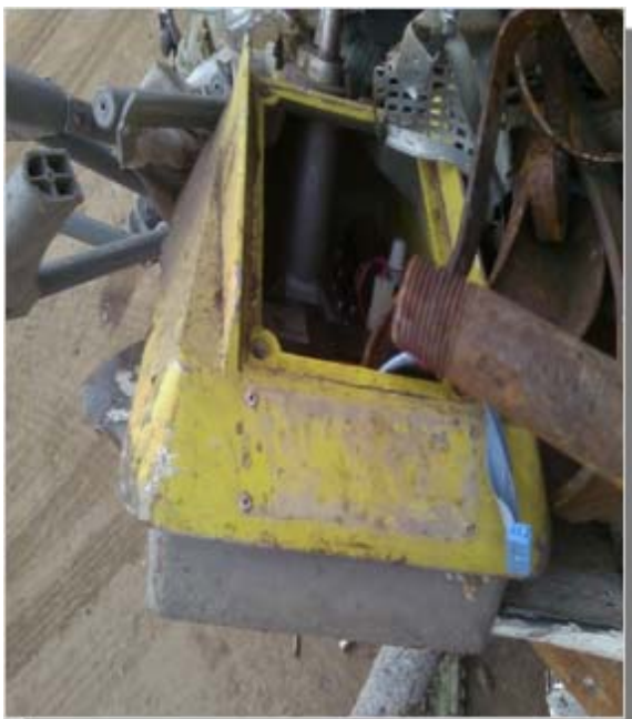
Damaged Portable Gauge
