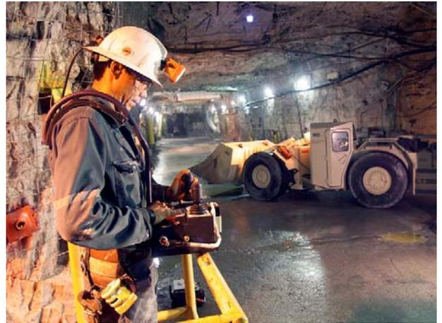
Figure 3: To decrease radiation exposure, a Cameco employee operates a remote-controlled truck to retrieve uranium ore from an underground extraction chamber at the McArthur River mine.
